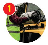
Replace empty cylinder with new full cylinder
