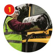
Replace empty cylinder with new full cylinder
