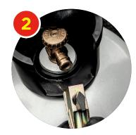
Connect the on truck LPG adaptor to the cylinder valve
