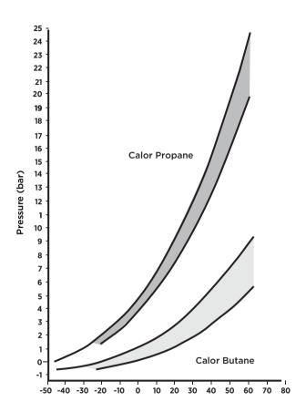
**Temperature** Vapour Pressures of Calor Butane and Calor Propane
